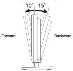
• The unit can be tilted up to 10 degrees forward and 15 degrees backward.
